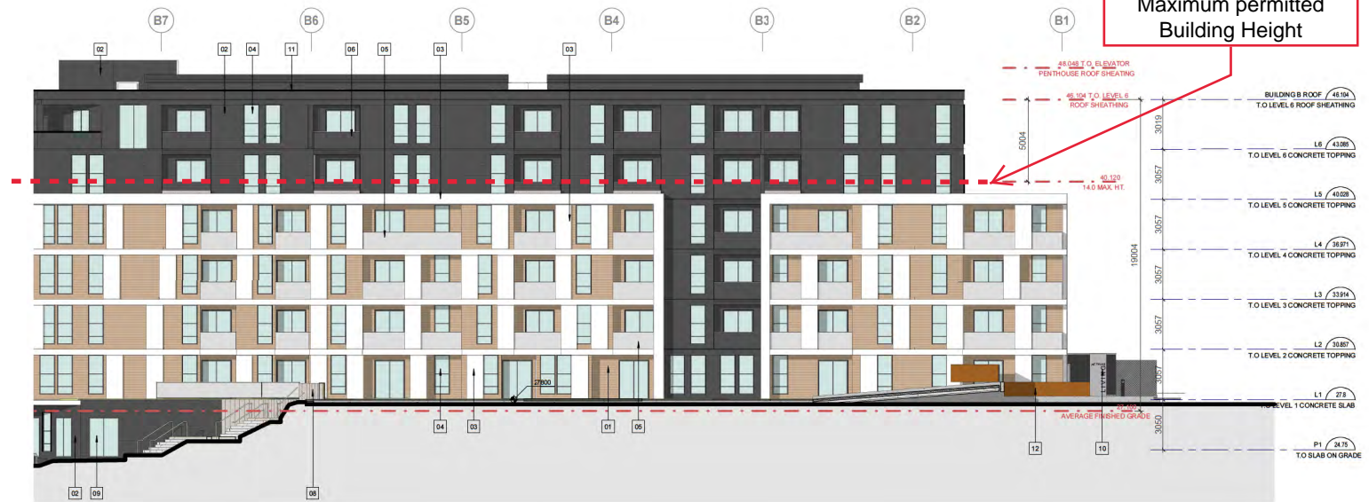
1 | ELEVATION - BUILDING B - GARDEN COURT SCALE: 1:125
